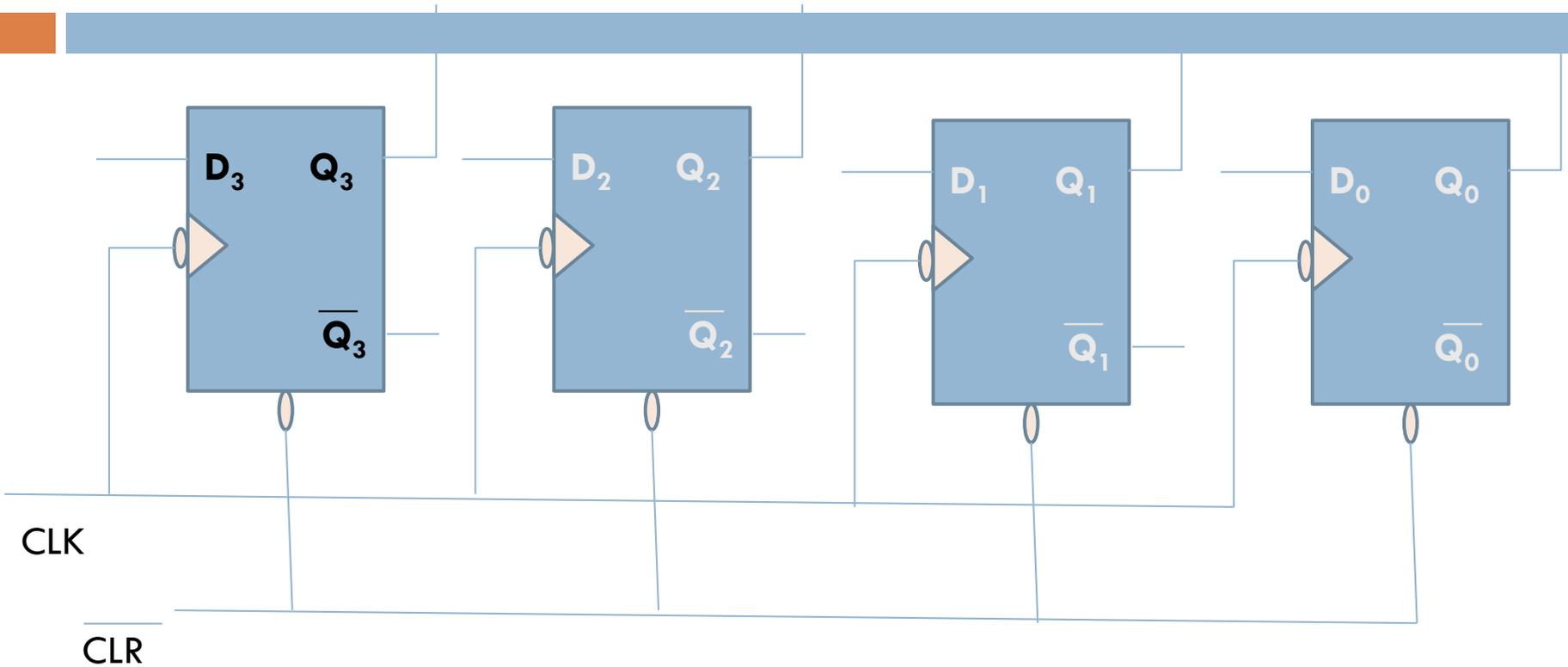
Data inputs are given at the D inputs of the flipflops.
